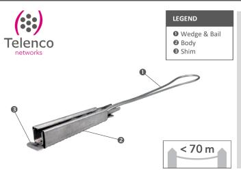
The Telenco® ODWAC and ODWAC XL clamps are designed for the dead-ending of aerial flat drop cables deployed on telecommunications networks where spans do not exceed 70m.
